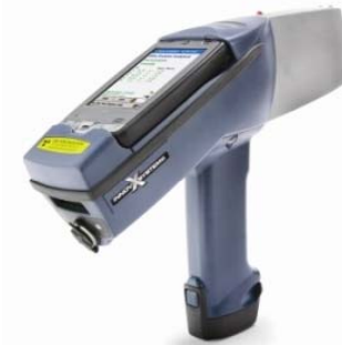
2002: Innov-X Alpha 1 st handheld with x-ray tube source
