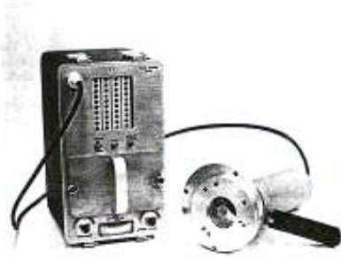
1967:TN 9200 1 st commercial field portable XRF; used non-dispersive scintillation detectors with x-ray filters
