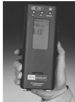
1994:NITON XL-309 1 st one piece, handheld XRF with real-time digital signal processing and silicon PIN diode detectors
